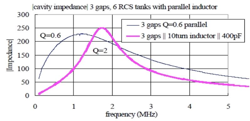
Fig. 5:  $Q_x=2$  at 1.7MHz with parallel inductor
