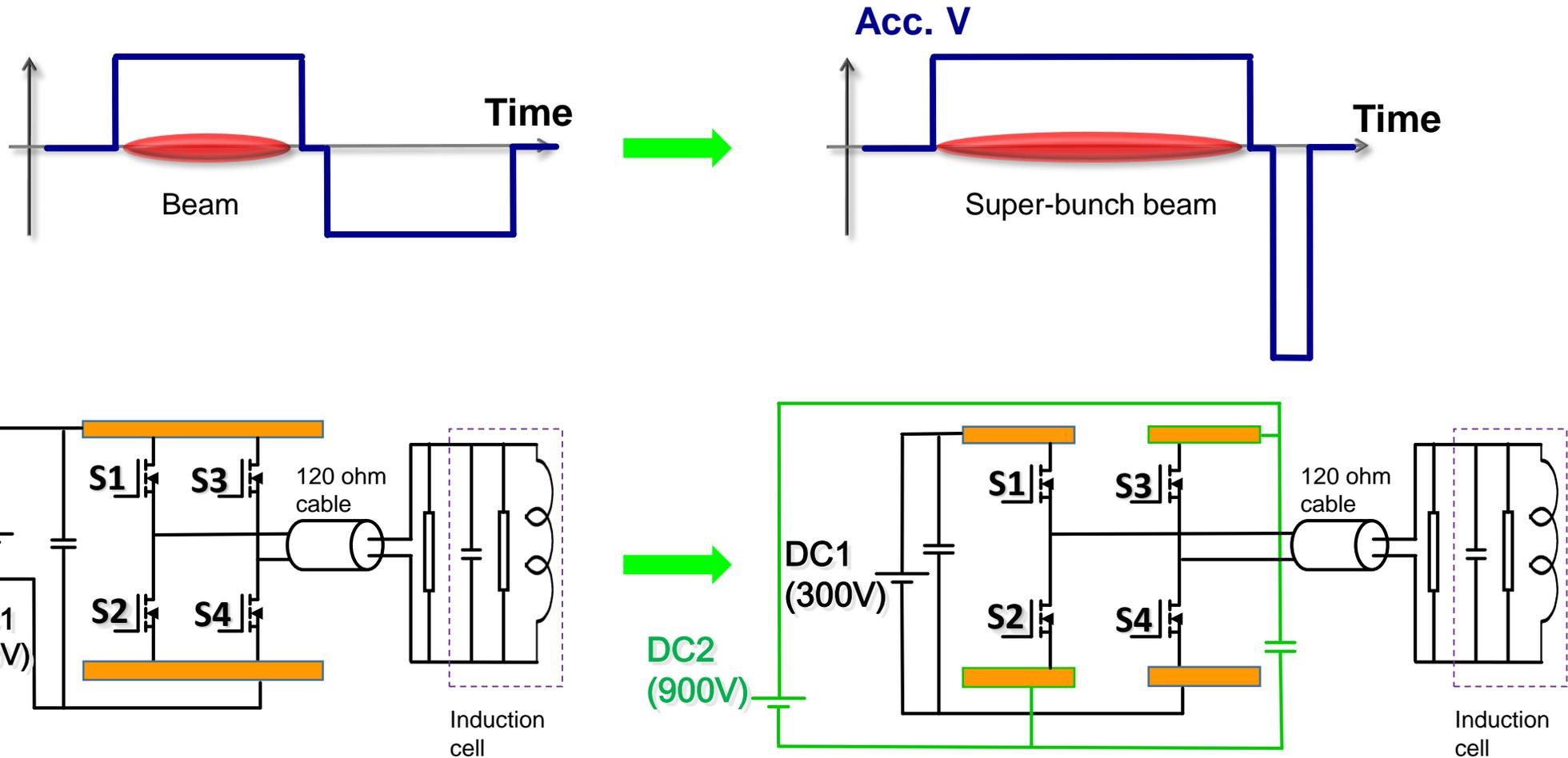
Different voltages are applied to positive and negative pulses.
