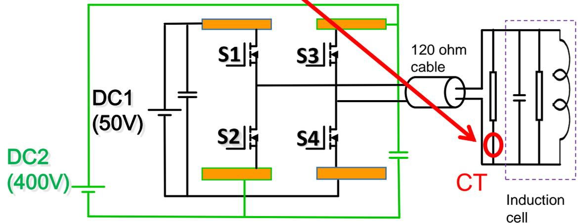
Asymmetric pulses can be generated with bridge circuits easily.
