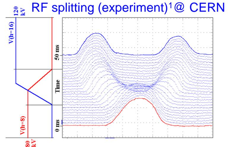
Figure 1: Beam pick-up signal and RF voltages during splitting at 3.57 GeV/c in the PS.
