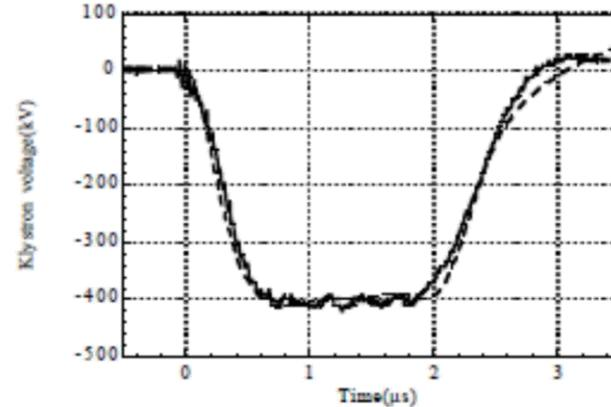
Figure 6. Output pulse waveform at the kly
