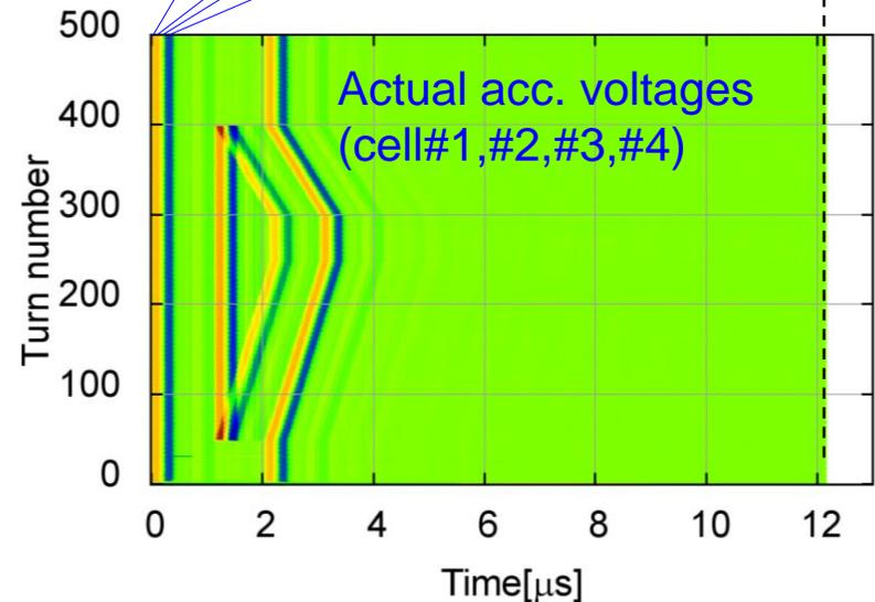
This FPGA code can generate arbitral pulse timings at each cell (Max.5) in each turn (Max.5000). Therefore everyone can program each arbitral pulse easily and flexibly.
