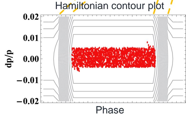
Separate function can create a longer bucket  $\Rightarrow$  Diminishing space charge effect. 6
