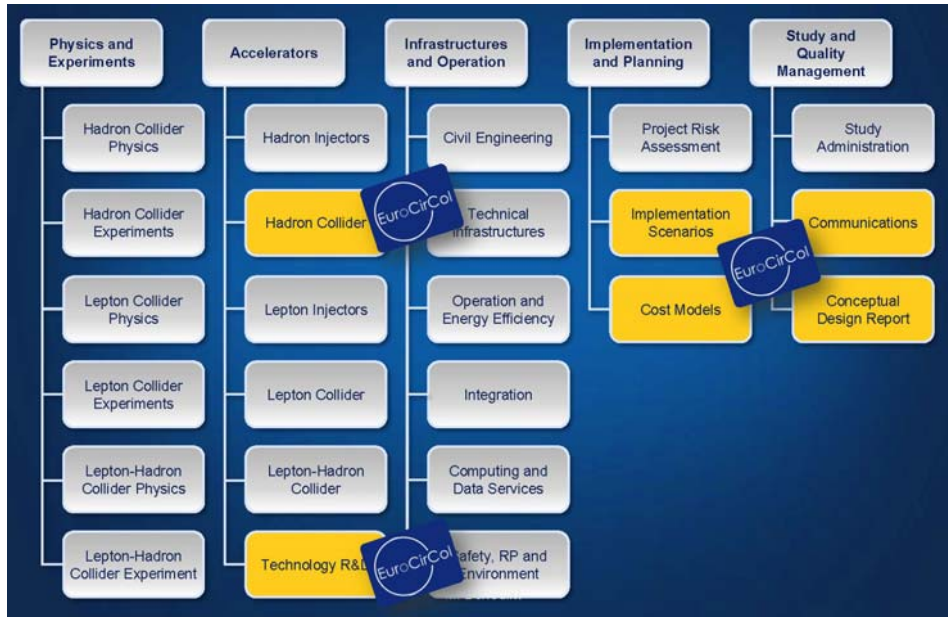
Figure 11: Work breakdown structure of global FCC study; highlighted in orange are the parts (partly) addressed by the HORIZON 2020 EuroCirCol project (Courtesy J. Gutleber).
