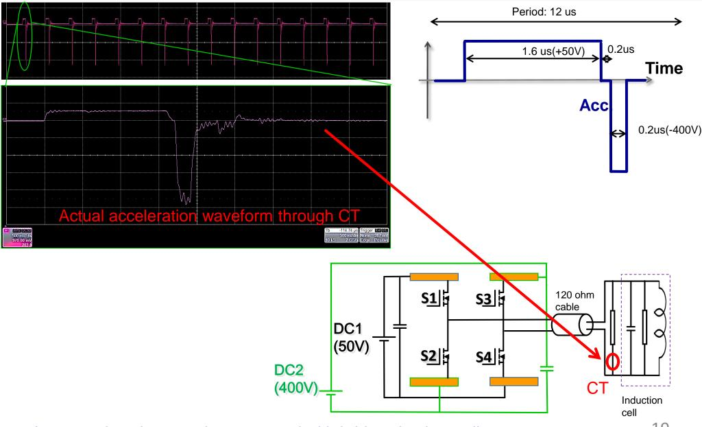
Asymmetric pulses can be generated with bridge circuits easily.
