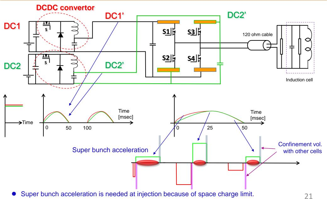
• Maximum voltage should be reduced because of difficulty of high-voltage and MHz switching.
