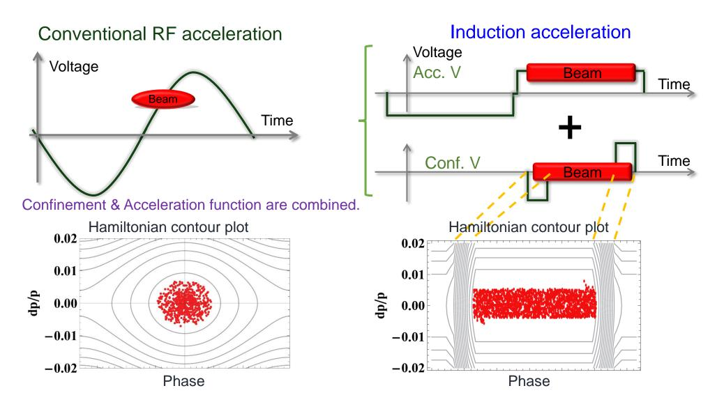
Separate function can creates a longer bucket  $\Rightarrow$  Diminishing space charge effect. 6
