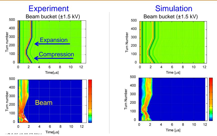
The beam motion of the experiment is reproduced in the simulation macroscopically. Therefore it is easy to design the beam length and quantity.
