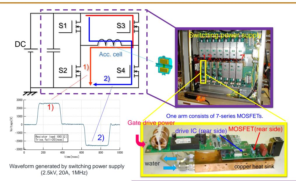
Next generation of SPS: K.Okamura, *et al*, MOPME068 in IPAC'14 "SiC-JFET Switching Power Supply toward for Induction Ring Accelerators"
