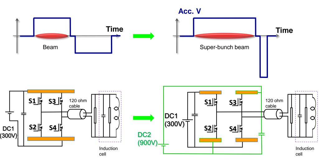
Different voltages are applied to positive and negative pulses.
