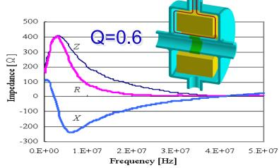
MA cavity with low Q is the same of induction cavity.
