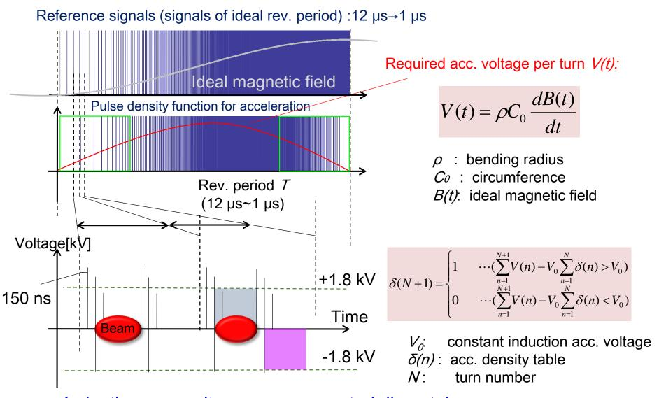
Induction acc. voltages are generated discretely in order to give required acc. voltage spuriously.
