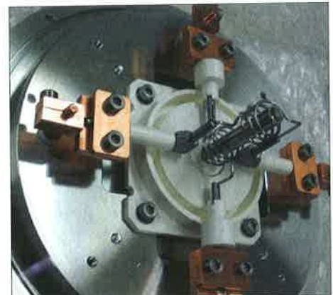
Fig. 1. The newly developed surface ion source (the grey tantalum tube in the centre of the photo surrounded by two heating filaments) installed in the JAEA-ISOL system at the JAEA Tandem accelerator. (Image credit: JAEA.)
