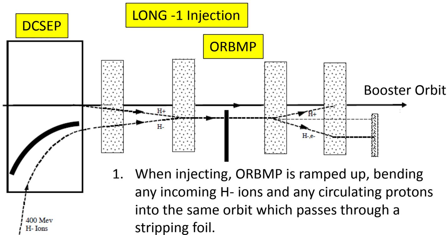
1. When injecting, ORBMP is ramped up, bending any incoming H<sup>-</sup> ions and any circulating protons into the same orbit which passes through a stripping foil.
