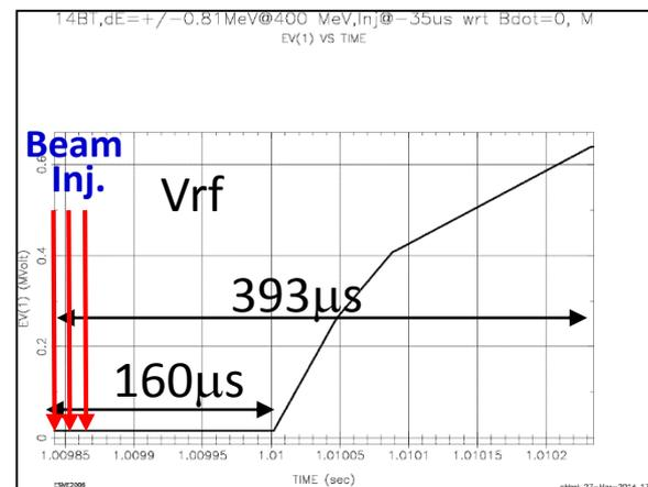
**Issues:** A limited time for Beam Capture. RF manipulations are non-adiabatic at capture ←  $\sim 50\%$  emittance dilution,  $\sim 10\%$  beam loss
