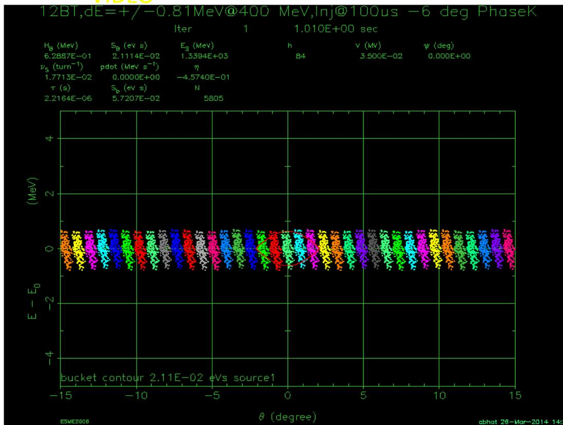
**Because of small emittance at capture acceleration needs less rf voltage**
