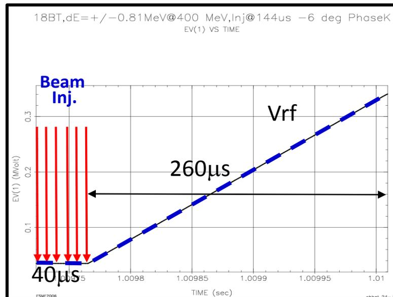
Since we impose  $\dot{P}=0$ , one demands  $\Delta B/B = \gamma_T^2 \Delta f/f$  during beam capture.
